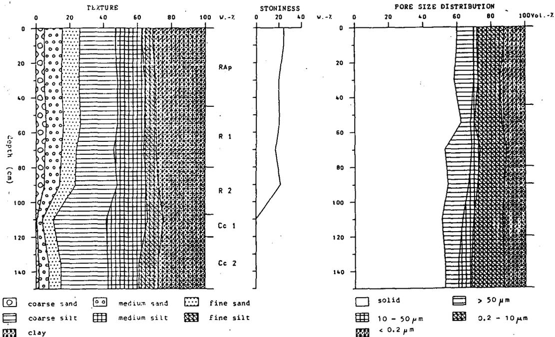
Fig. 1: Fuchsberg soil physical properties
